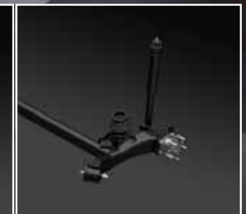
Torsion beam rear suspension with specially designed trailing arm
